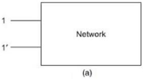
A **two-port network** is simply a network inside a black box, and the network has only two pairs of accessible terminals; usually one pair represents the input and the other represents the output. Such a building block is very common in electronic systems, communication systems, transmission, and distribution systems. The Figure(b) shows a two-port network, or a two terminal pair network, in which the four terminals have been paired into ports 1-1' and 2-2'.
