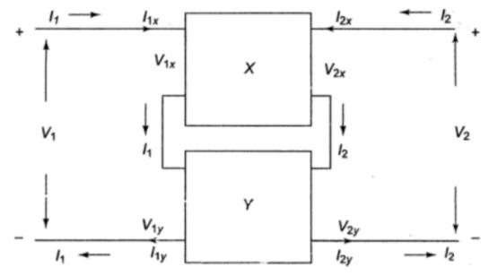
Let us consider two, two-port networks, connected in series as shown. If each port has a common reference node for its input and output, and if these references are connected together then the equations of the networks X and Y in terms of Z parameters are
