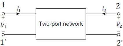
The terminals 1-1' together constitute a port. Similarly, the terminals 2-2' constitute another port. Two ports containing no sources in their branches are called passive ports; among them are power transmission lines and transformers. Two ports containing sources in their branches are called active ports. A voltage and current assigned to each of the two ports.
