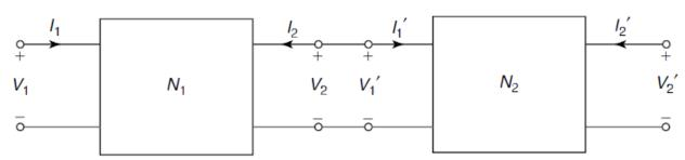
Let  $A_1,B_1,C_1,D_1$  be the transmission parameters of the network  $N_1$  and  $A_2,B_2,C_2,D_2$  be the transmission parameters of the network  $N_2$ .
