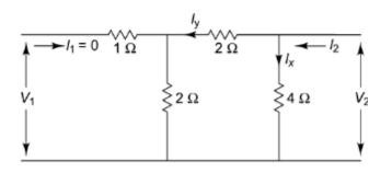
13) Find the hybrid parameters for the two-port network of Fig.
