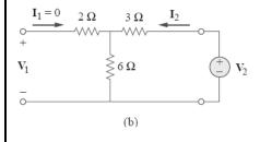
To obtain  $\mathbf{h}_{12}$  and  $\mathbf{h}_{22}$ , we open-circuit the input port and connect a voltage source  $\mathbf{V}_2$  to the output port as in Fig.(b). By voltage division,
