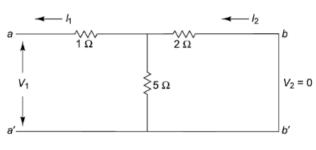
8) Obtain ABCD parameters for the network shown in Fig
