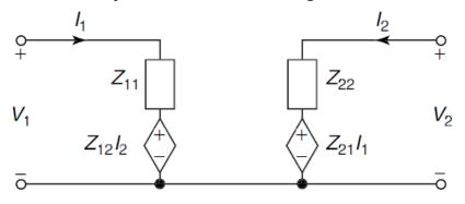
The network is to be reciprocal if  $Z_{12} = Z_{21}$ The network is to be symmetrical if  $Z_{11} = Z_{22}$
