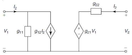
The network is to be reciprocal if  $g_{12} = -g_{21}$ The network is to be symmetrical if  $g_{11}g_{22} - g_{12}g_{21} = 1$
