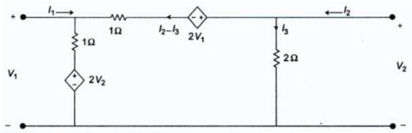
Let  $I_3$  be the current through  $2\Omega$ . KVL to the outer loop.
